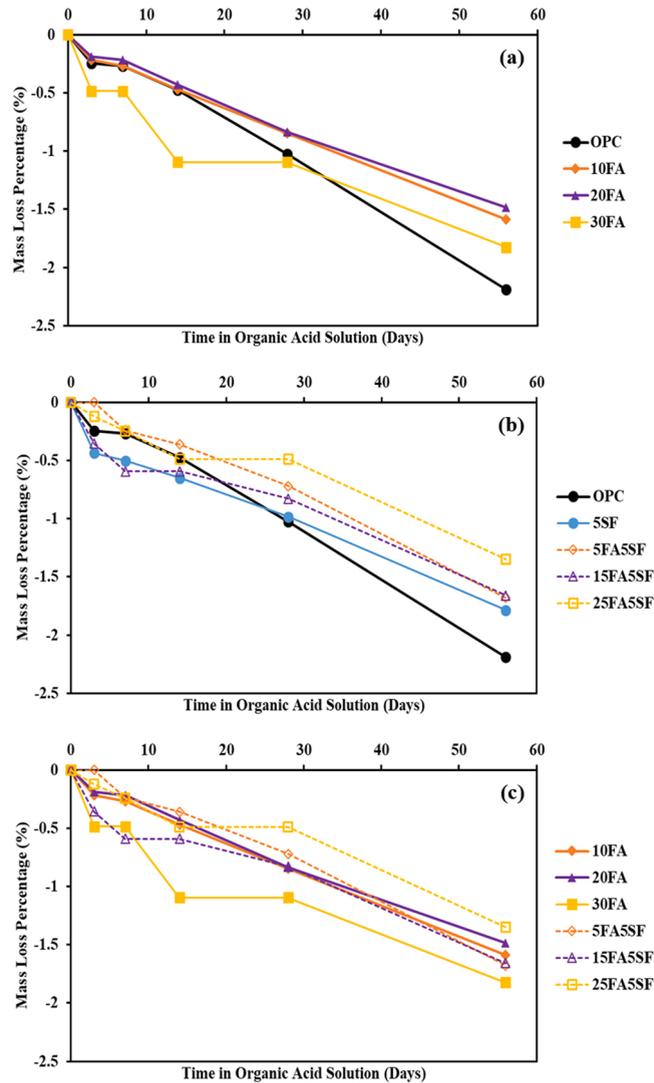
**Fig. 8.** Age-dependent mass loss of mortar due to organic acid corrosion; (a) FA system, (b) FA-SF system and (c) comparison of the similar pozzolan content.
