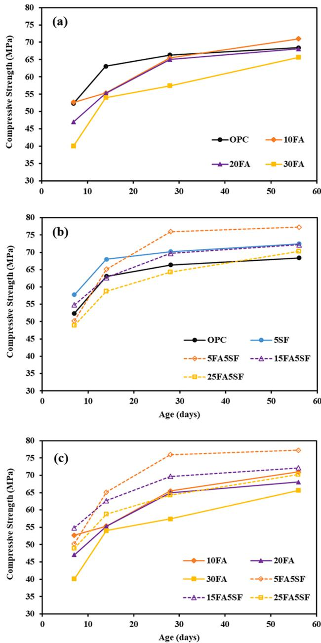
Fig. 7. Age-dependent compressive strength development of concrete; (a) FA system, (b) FA-SF system and (c) comparison of the similar pozzolan content.
