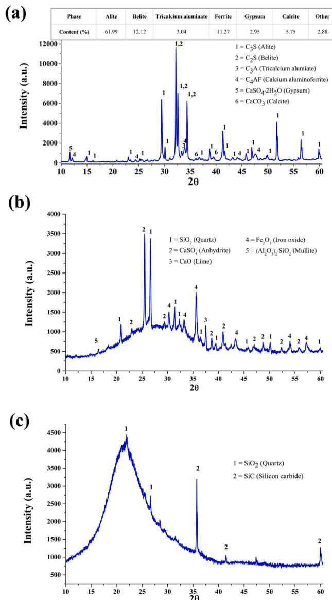
**Fig. 3.** X-ray diffractometry patterns of raw materials; (a) OPC, (b) fly ash and (c) silica fume.
