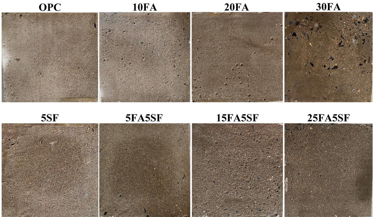
**Fig. 10.** Surface of test specimens after 5 cycles of wet-dry condition switching system in an organic acid solution cooperating with abrasion corrosion test.
