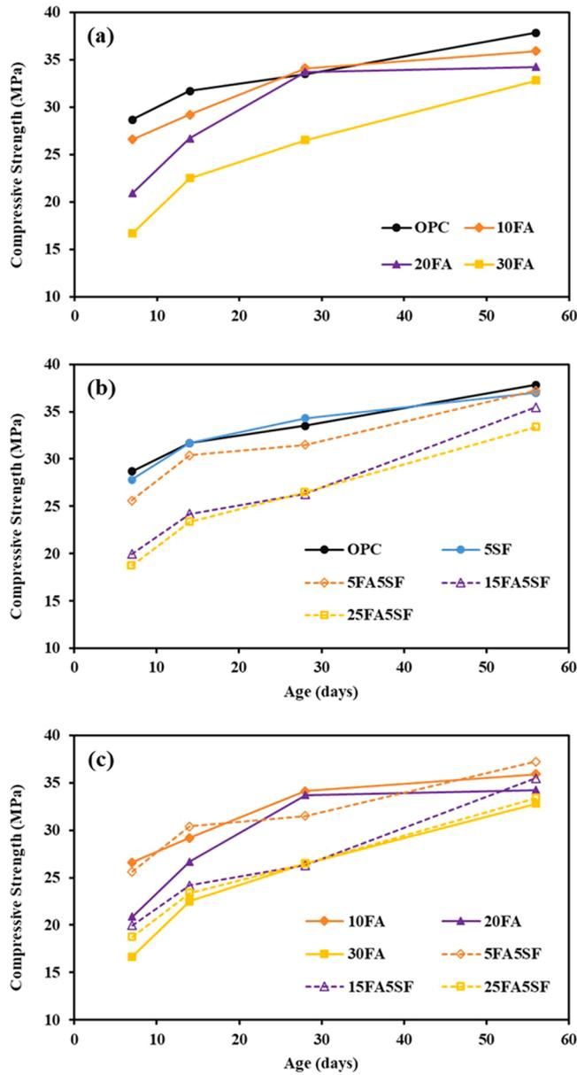
Fig. 6. Age-dependent compressive strength development of mortar; (a) FA system, (b) FA-SF system and (c) comparison of the similar pozzolan content.
