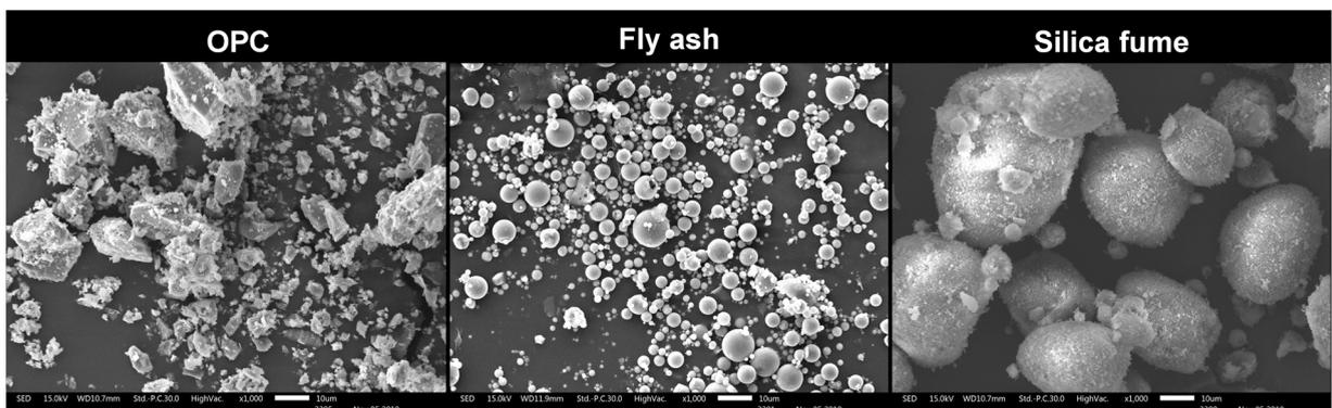
Fig. 2. SEM images of OPC, fly ash, and silica fume.
