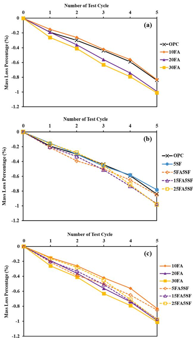
Fig. 11. Mass loss of concrete due to combination of organic acid corrosion and abrasion corrosion; (a) FA system, (b) FA-SF system and (c) comparison of the similar pozzolan content.
