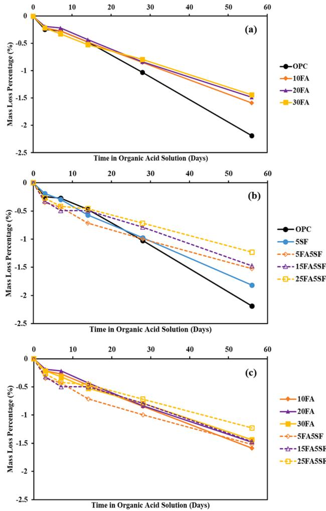
Fig. 9. Age-dependent mass loss of concrete due to organic acid corrosion; (a) FA system, (b) FA-SF system and (c) comparison of the similar pozzolan content.
