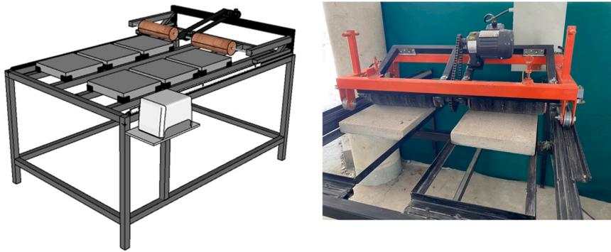
Fig. 5. Abrasion corrosion testing machine.
