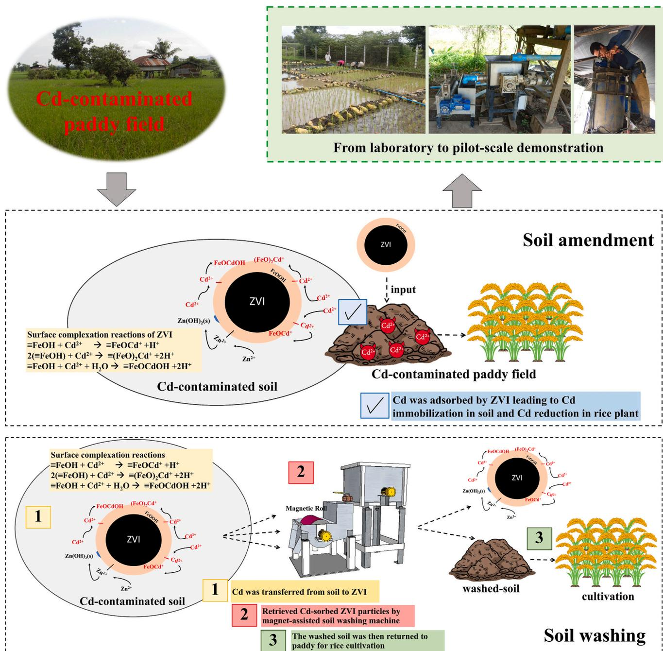
Fig. 1. Zerovalent iron for stabilizing cadmium via soil amendment and for removal from soil via magnet-assisted soil washing.
