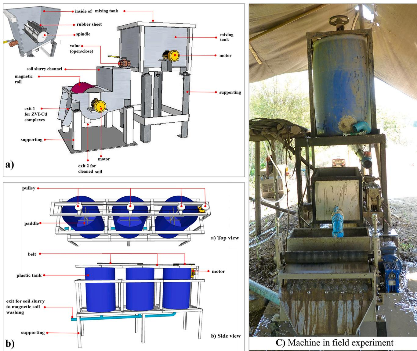
Fig. 2. a) Magnet-assisted soil washing and b) soil slurry mixing tank prototype in c) field experiments.
