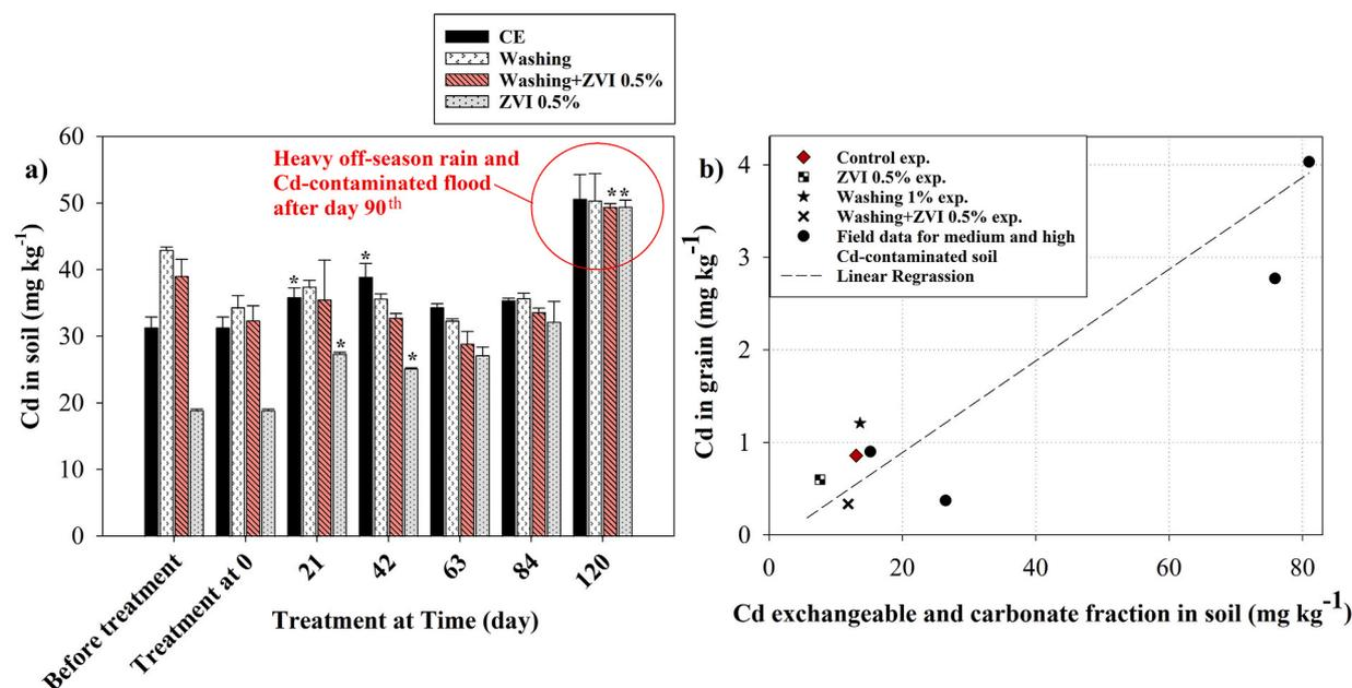
Fig. 5. Results of the experiments including a) change in cadmium concentration in soil and b) hypothetical cadmium concentration in treatment with/without soil amendment and soil washing. Statistical significance ( $p$  value < 0.05) for each treatment vs. CE, or between conditions, is indicated by an asterisk (\*).
