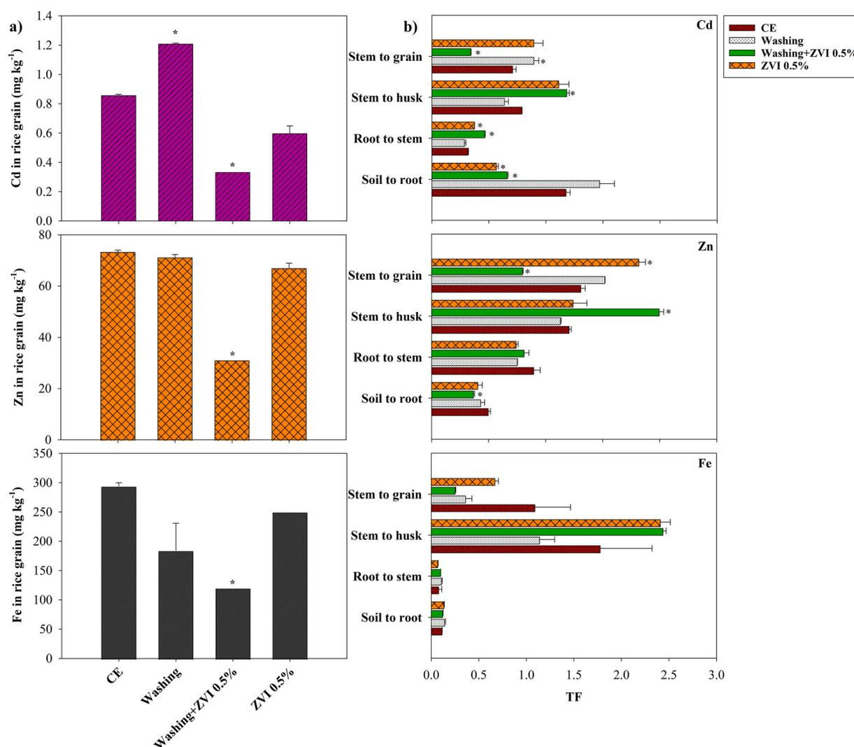
**Fig. 4.** Results of the experiments including a) cadmium level and b)  $TF$  in rice grain at harvest time in soil. Statistical significance ( $p$  value < 0.05) for each treatment vs. CE, or between conditions, is indicated by an asterisk (\*).
